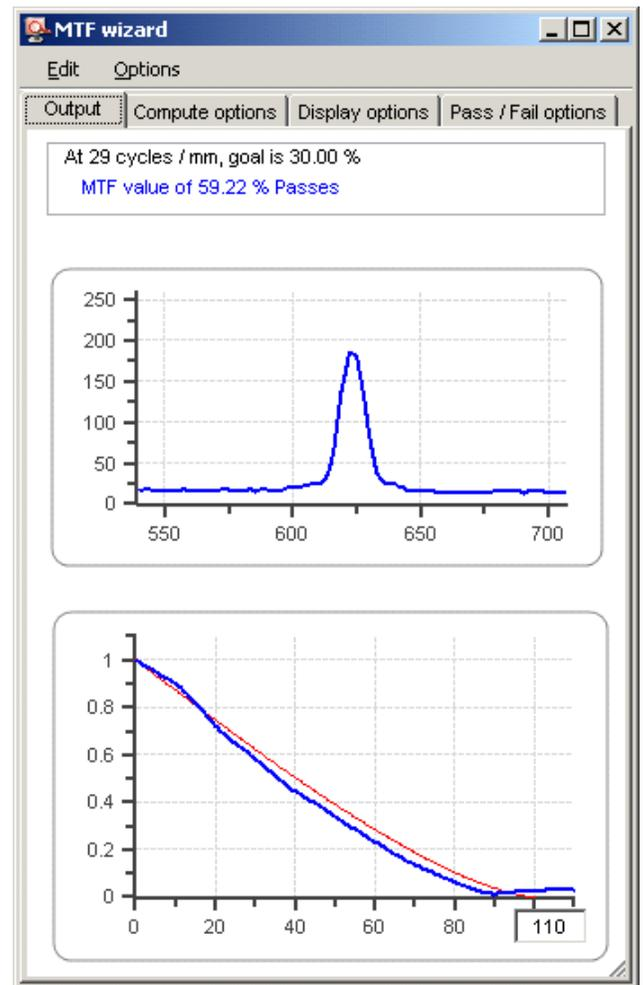
Figure 3: NV3, 12.8mm f/1 optical performance measurements
