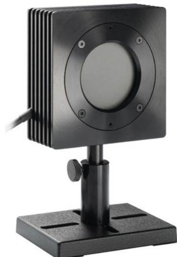
cumbersome, water-cooled devices,” said Ephraim Greenfield, CTO of Ophir Photonics Group. “Today’s lasers can be switched on and off precisely, delivering a rectangular pulse of energy. Our new, compact non-water cooled laser sensors use these short pulses of 0.1 to 1 sec to make laser power measurements up to 8000W or higher.”
