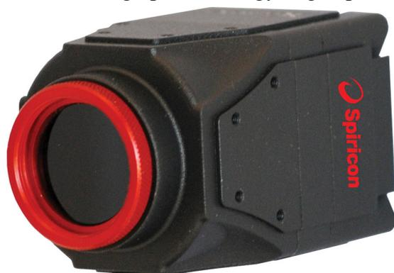
lower noise electronics and a unique thermal management technology that delivers a more stable background; this results in more consistently accurate results.
