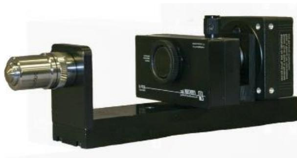
Figure 6. Photograph of near field beam profiling system
