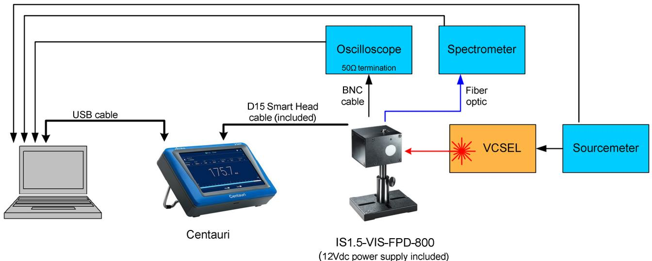
**Figure 1. Schematic diagram of a complete VCSEL characterization system build around the IS1.5-VIS-FPD-800**
