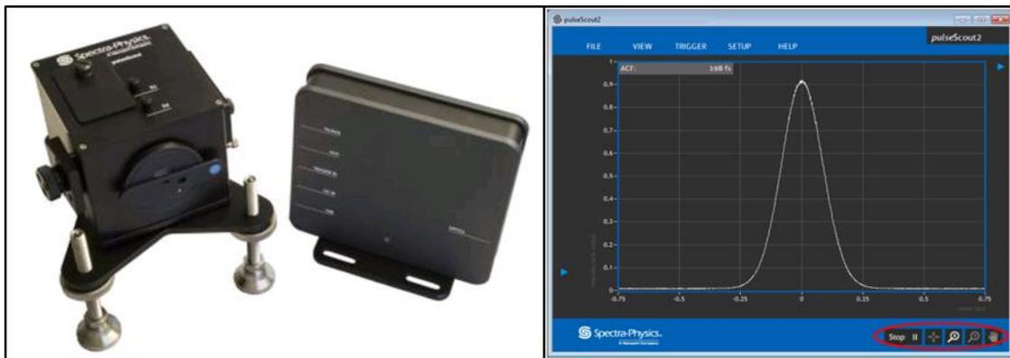
**Figure 2. Left: PulseScout2 Autocorrelator from Newport. Right: Autocorrelation trace of a 198 femtosecond pulse.**
