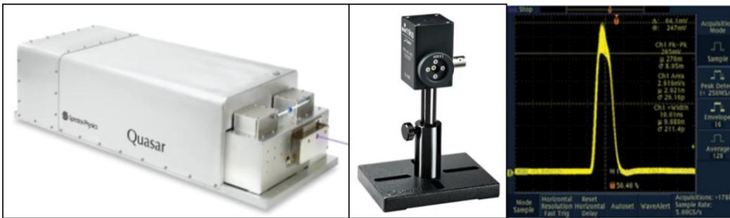
**Figure 4. Spectra Physics Quasar Laser, Ophir FPD-VIS-300 and a typical 10 ns pulse profile.**
