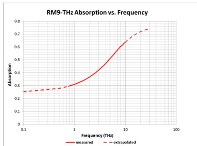
Figure 2. Absorption spectra of RM9-THz
