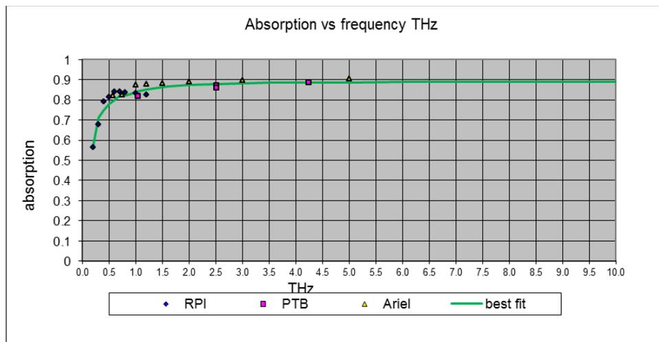
Figure 1. Absorption spectra of 3A-P-THz
