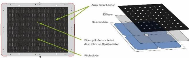
Figure 3: Components and structure of the Ophir FluxGage system
