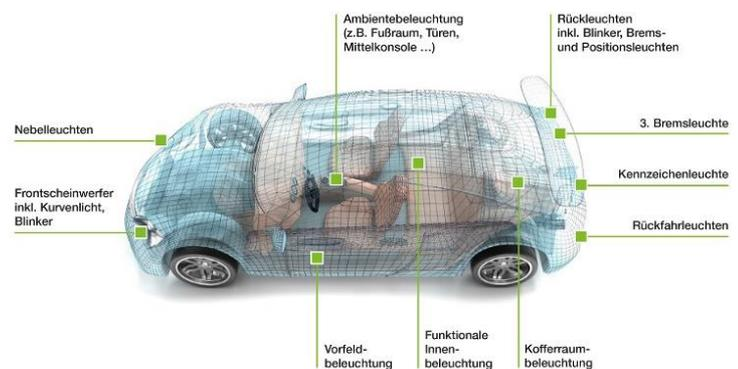
Figure 1 (car with lettering based on photo © iStock.com/alex-mit): LED technology is already being used widely in today's vehicles, as the image shows. Autonomous cars will only further push the envelope for new applications.
