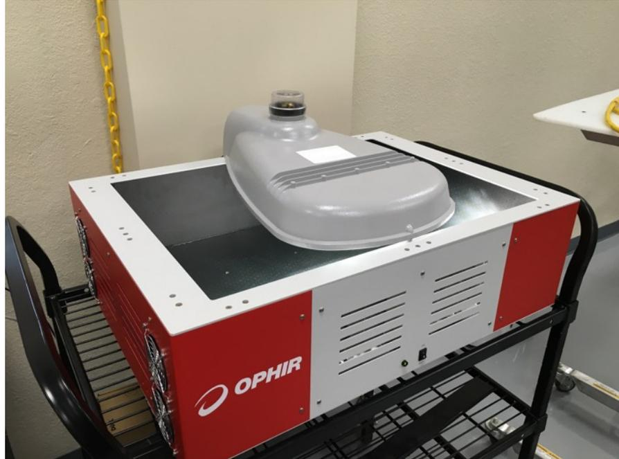
process calls for the lamp to be positioned onto the FluxGage, turned on, measurements take, and quality data is immediately compared against standards.
