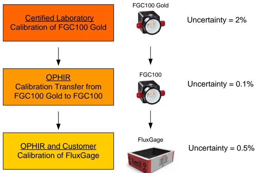
Figure 3. FluxGage calibration chain
