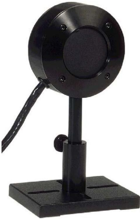
*50 mm diameter pyroelectric head.*
