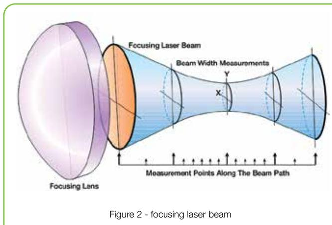
Figure 2 - focusing laser beam
