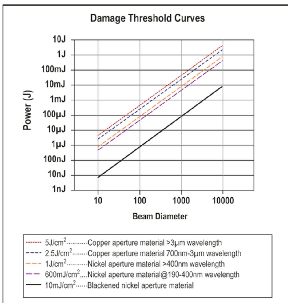
Fig. 1: Energy Damage Thresholds for various wavelength ranges and slit materials
