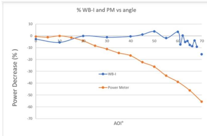
Figure 2. Linearity of Ophir WB-I energy distribution for angled light compared to the measurements of a photodiode sensor.
