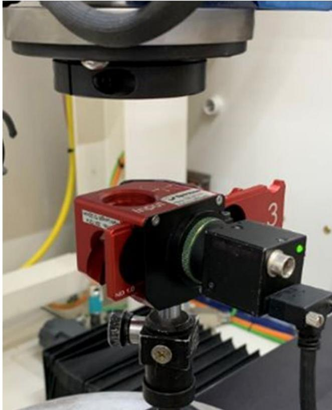
*Figure 7. Ophir LBS-300HP-NIR and camera measuring 5kW Fiber Laser.*
