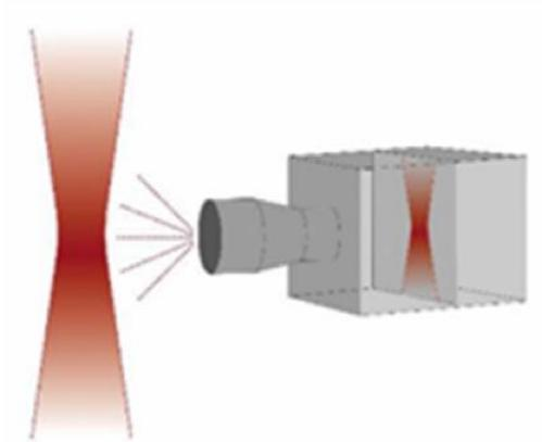
Figure 3. The Ophir BeamWatch AM is a 3D Additive Manufacturing Metal Powder Printing laser beam diagnostics device.
