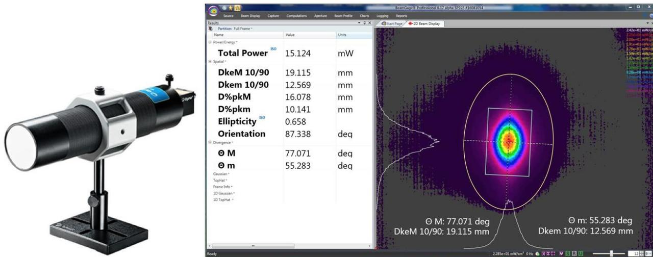
Figure 1. Ophir Wide Beam Imager and BeamGage profiling software.
