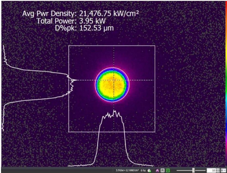
Figure 6. Beam profile of focused 4kW Fiber Laser - Average Power Density 21.4MW/cm<sup>2</sup>.
