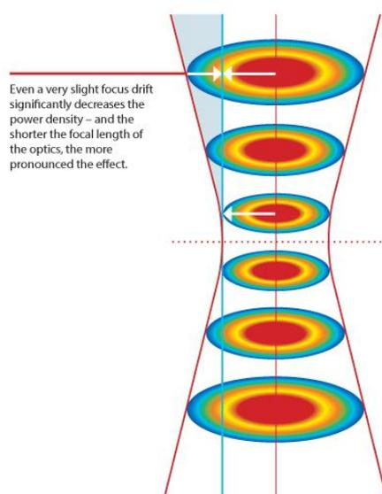
Fig. 2: A change in the focus position changes the power density and thus the entire laser process.
