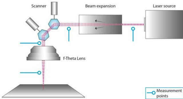
Fig. 2: Structure of a 2-axis galvo system: Measurements between the components provide information about their function.
