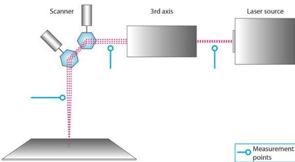
Fig. 3: Construction of a 3-axis galvo system: Here, too, measurements can be taken between the components.
