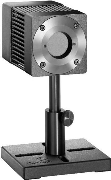
Fig. 4: Example of a 4-quadrant sensor, the Ophir F150A-BB-26-PPS
