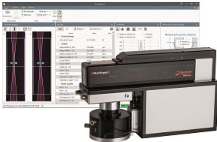
*Fig. 2: Ophir BeamWatch Integrated Short Distance delivers key beam parameters such as focal shift in real-time*
