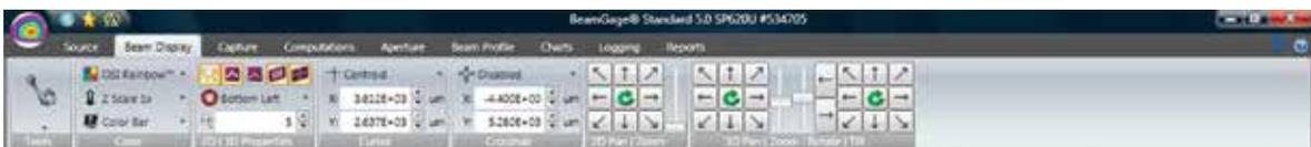
Some of the Beam Display options (Display access options under the Tools tab on the left).
