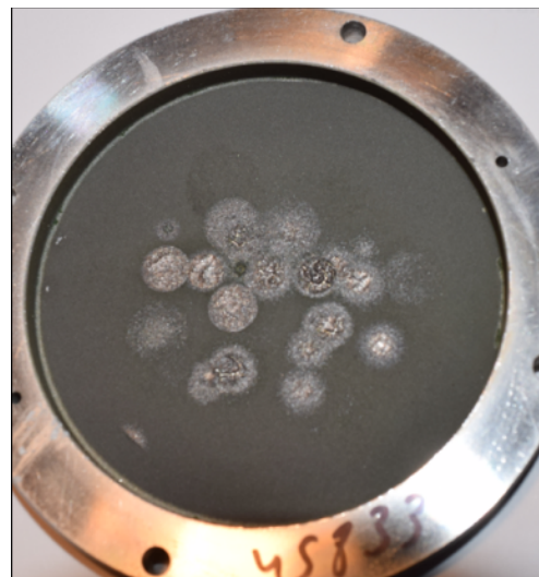
Figure 2. Disc Condition: Damaged, heavily pitted with coating ablated — inaccurate measurements, must be replaced.
