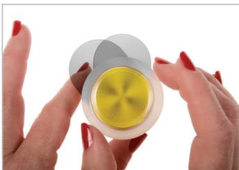
**Step 7:** Twist the top cleaning holder 90° left to view & inspect the lens for stress
