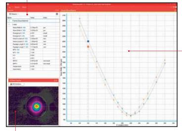
This window displays the 2D or 3D beam profile of the currently measured point in the beam propagation curve. This image enables visual intuitive verification of the beam profile behavior through focus. After each run the user can click any individual measured point and observe the beam profile. Outlying or anomalous points can be automatically or manually excluded from the curve fit calculations for more accurate results.
