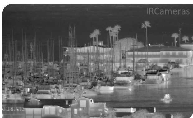
Image 1: IR thermal image taken with SupIR 28-850mm f/5.5 SXGA format continuous zoom lens from 3.6km distance, integrated by IR Cameras infrared imaging system.
