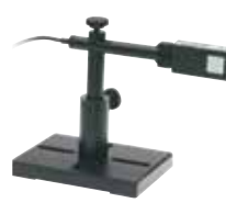
PD300 with filter installed
