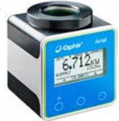
The Ariel measures high power industrial lasers of up to 8kW by measuring the energy of a short exposure to this power. The laser is set to deliver a pulse of from 0.05 to several seconds. It then measures the energy and duration of the
