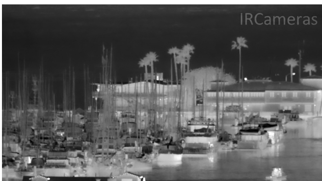
Image 1: IR thermal image taken with SupIR 28-850mm f/5.5 HD format continuous zoom lens from 3.6km distance, via IR cameras infrared imaging system.
