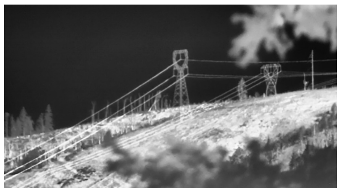
Image 2: IR thermal image taken with SupIR 16-180mm f/3.6 VGA format continuous zoom lens from 6.1km distance, via Ventus Micro by Sierra Olympia Technologies Inc.
