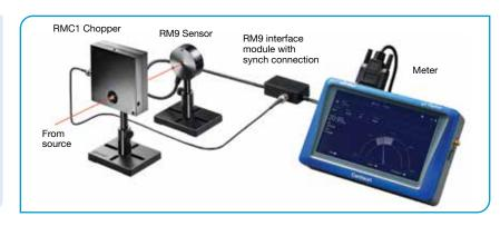
The RM9 series Radiometers use a pyroelectric or photodiode sensor in conjunction with chopped CW or quasi CW radiation, using a digitally synthesized lock-in amplifier to reduce external noise to a minimum. The signal is passed through the 18Hz chopper and the chopped signal is detected by the sensor. All signals not at this 18Hz frequency
