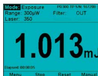
Exposure measurement (energy summing) with photodiode sensor.
