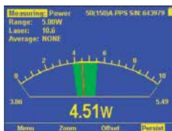
Analog needle display of power Persistence and min/max tracking.
