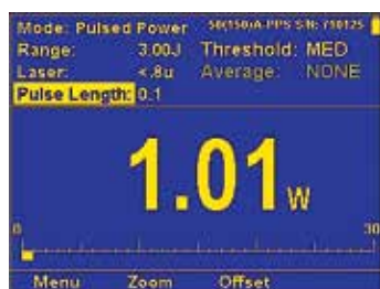
Power measurement of laser pulse. For use with high-power pulsed lasers.
