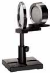
Beam splitter installed – reflected beam on sensor
