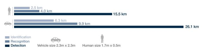
Assumptions: 1280 detector | TRM4 model | Day mode | 0.7µm to 1.7µm spectral range | 25Hz frame rate | Overcast daylight irradiance | 0.2 path radiance factor | 0.2km<sup>-1</sup> atmospheric attenuation coefficient | 50% detection probability | Human and vehicle target 50% reflectivity | 15% background reflectivity
