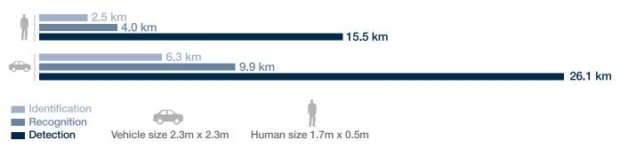
Assumptions: 1280 detector | TRM4 model | Day mode | 0.7µm to 1.7µm spectral range | 25Hz frame rate | Overcast daylight irradiance | 0.2 path radiance factor | 0.2km<sup>-1</sup> atmospheric attenuation coefficient | 50% detection probability | Human and vehicle target 50% reflectivity | 15% background reflectivity
