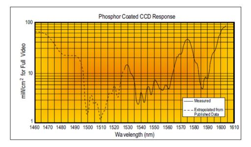
Figure 4, The absorption curve for the Phosphor coated cameras showing higher efficacy of phosphor coating converting 1550nm beam than 1400nm or 1600nm beam into visible light, detected by the sensor
