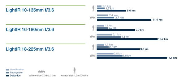
Note: Calculation used are based on "Johnson Criteria" | Real world performance may vary depending on the weather conditions
