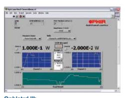
OphIstrd.IIb Library supplied for use with the Dual-Channel LaserStar. Communication can be set to RS232 or GPIB and is based on NI-VISA.
