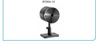
The BT50A-15 absorbs a laser beam that is inserted into the entrance aperture parallel to the unit's optic axis. The beam trap is designed that only a very small fraction of the light is backscattered. The BT50A-15 does not measure power. It is a beam trap only.
