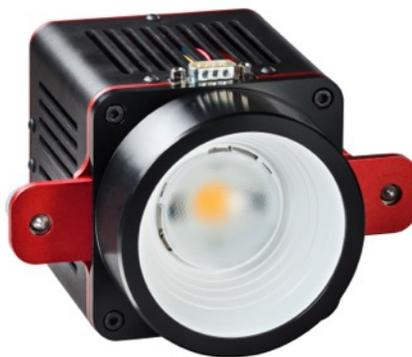
To ensure reliability, the FGC100 is calibrated at Ophir using a NIST-traceable source. The spectral flux data is provided on USB drive. The FGC100 controller includes an hour meter that indicates the total working time of the unit. After 50 hours, the FGC100 should be sent to Ophir for recalibration.
