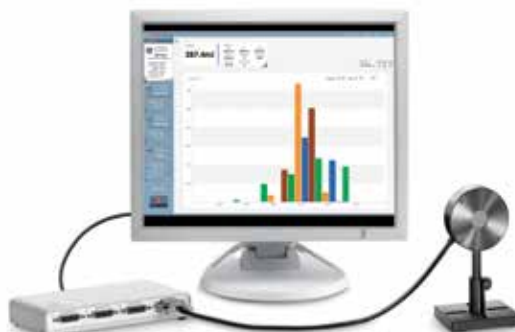
Pulsar-4 operating with StarLab software
