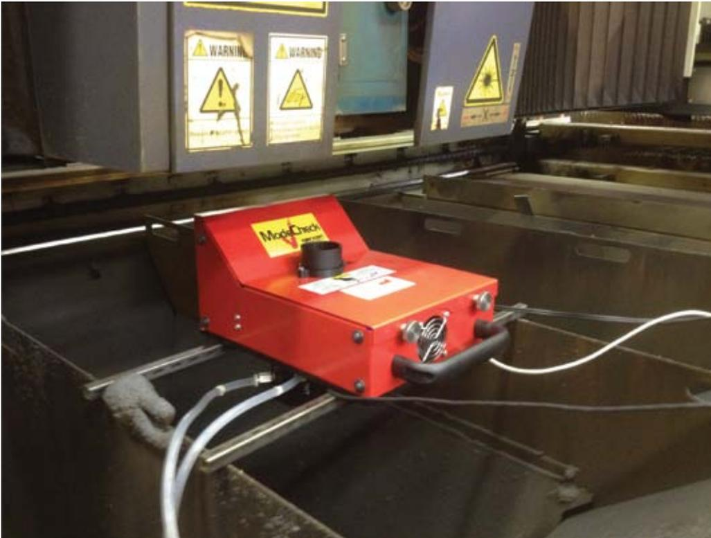
ModeCheck with optional MLA, profiling a CO<sub>2</sub> cutting laser with its processing head installed
