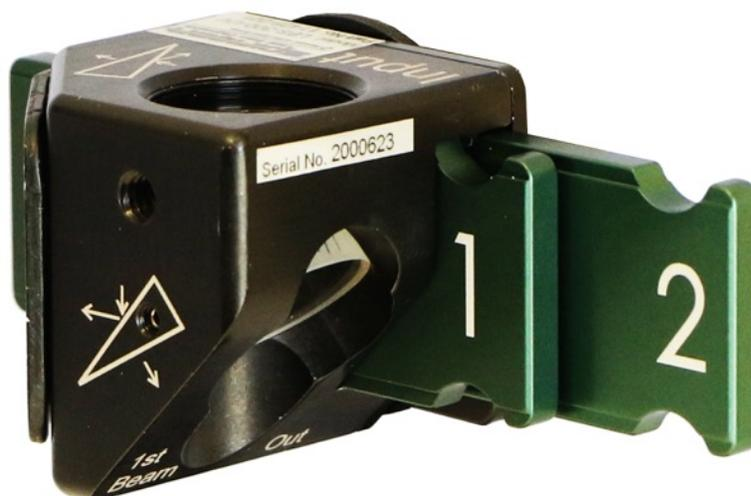
beam sampler with 0.01% passed on to the camera. The beam sampler provides a beam image that is polarization corrected to restore the polarization components of the original beam.
