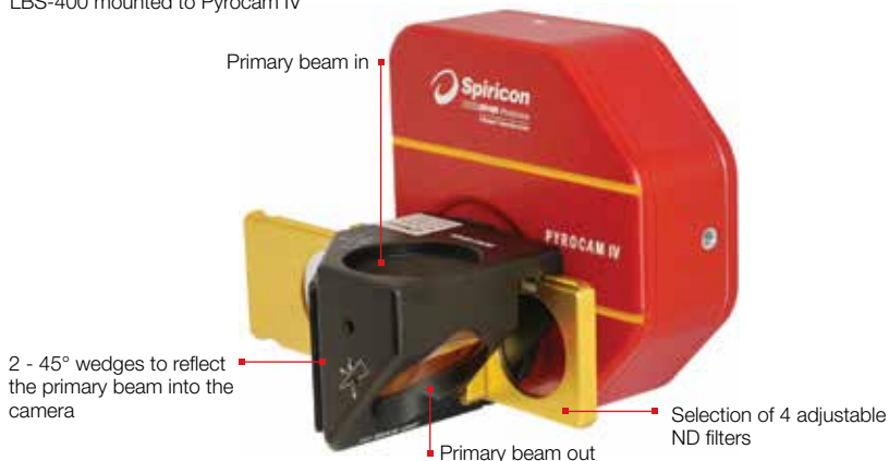
LBS-400 mounted to Pyrocam IV
