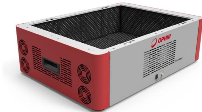
The **FluxGage** is an all-in-one photometric test system that uses  $2\pi$  (two pi) geometry. A spectrometer is incorporated for color measurement of the spectrum, CCT (correlated color temperature), CRI (color rendering index), Duv, and chromaticity. There is also a fast photodetector for flicker measurements. No fibers are needed.
