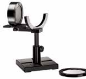
Beam Splitter removed – direct beam on sensor
