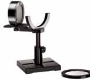
Beam Splitter removed – direct beam on sensor
