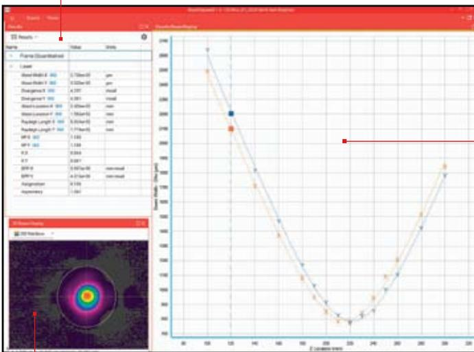
This window presents measurements of beam width vs. position for a given run. After measuring a few points, the software extrapolates a curve fit. The Xs and Ys represent individual measurement points. The solid lines present the best fit hyperbola of the beam propagation equation to the measured points. The  $M^2$  and other laser parameters are computed from the best fit hyperbola since it provides a smoothing of the data points.
