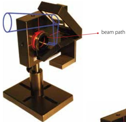
For converging beams a larger aperture splitter can be used either by itself or stacked (as shown)
