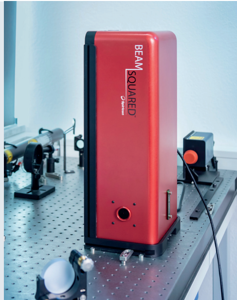
Fig. 2+3: Nearly every manufacturing step in building the laser is accompanied by measurements taken with the Ophir BeamSquared system.
