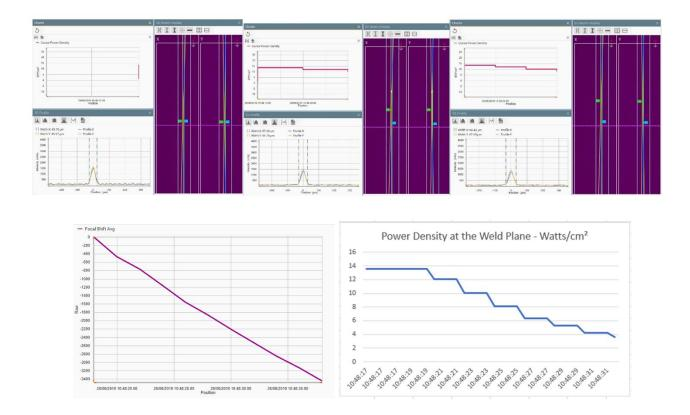
Figure 2. Chart laser power, 3-4 BeamWatch 2D graphs of focal shift, Chart of power density at weld plane.
