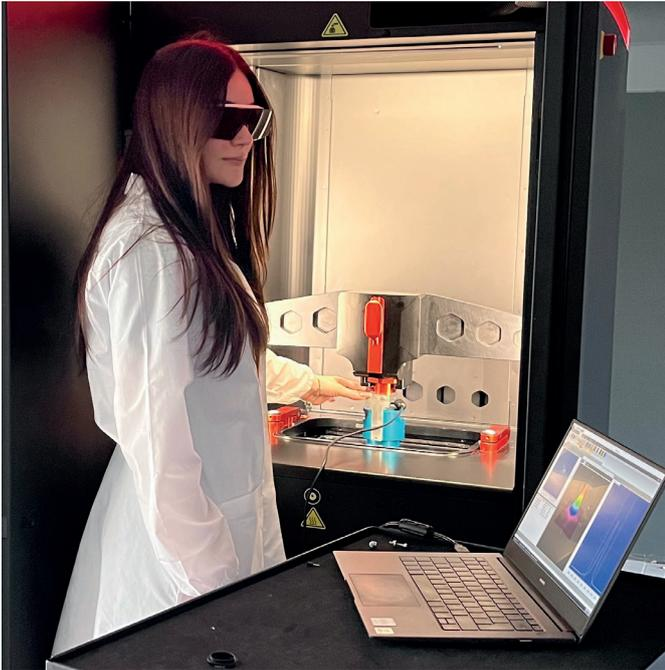
Figure 1: The Ophir NanoScan beam profiler is key to ensure the reproducibility in the AM process.
