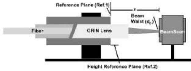
Fig. 3: Placing the profiler at the intended waist location allows the direct measurement of the focusing adjustments to the device
