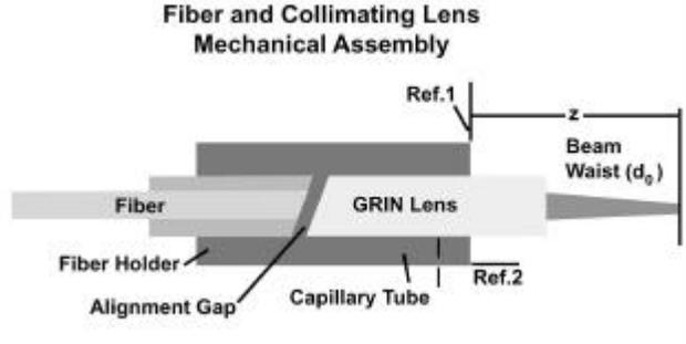
Fig 4: Optical device with characterized light beam as part of the part
