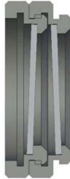
Filters are angled to reduce interference
