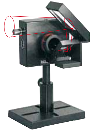
With large beam splitter mounted showing how to image converging beam
